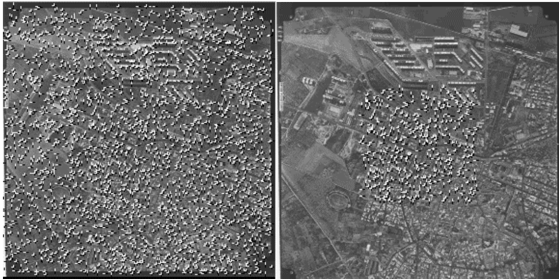
Fig. 2.4 – An aerial image with all the interest points extracted (secondary points, on the left) and with the primary points (on the right)
