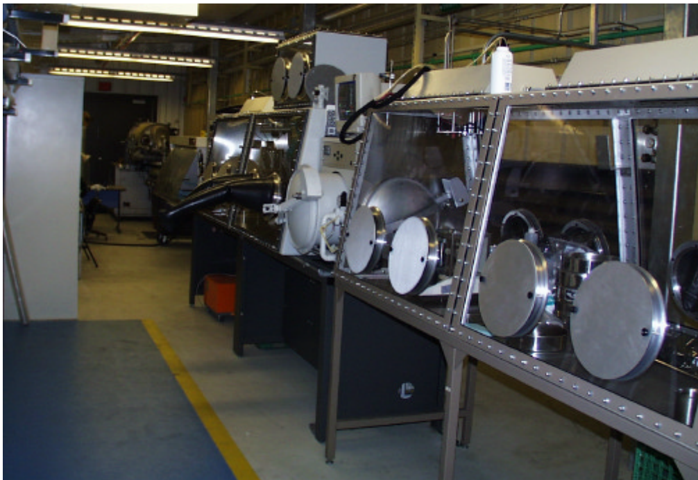
Figure 4-3 Argon controlled atmosphere glove box.. The water and oxygen level was continuously monitored and kept below few parts per million by an active getter bed through which the argon was flowed.
