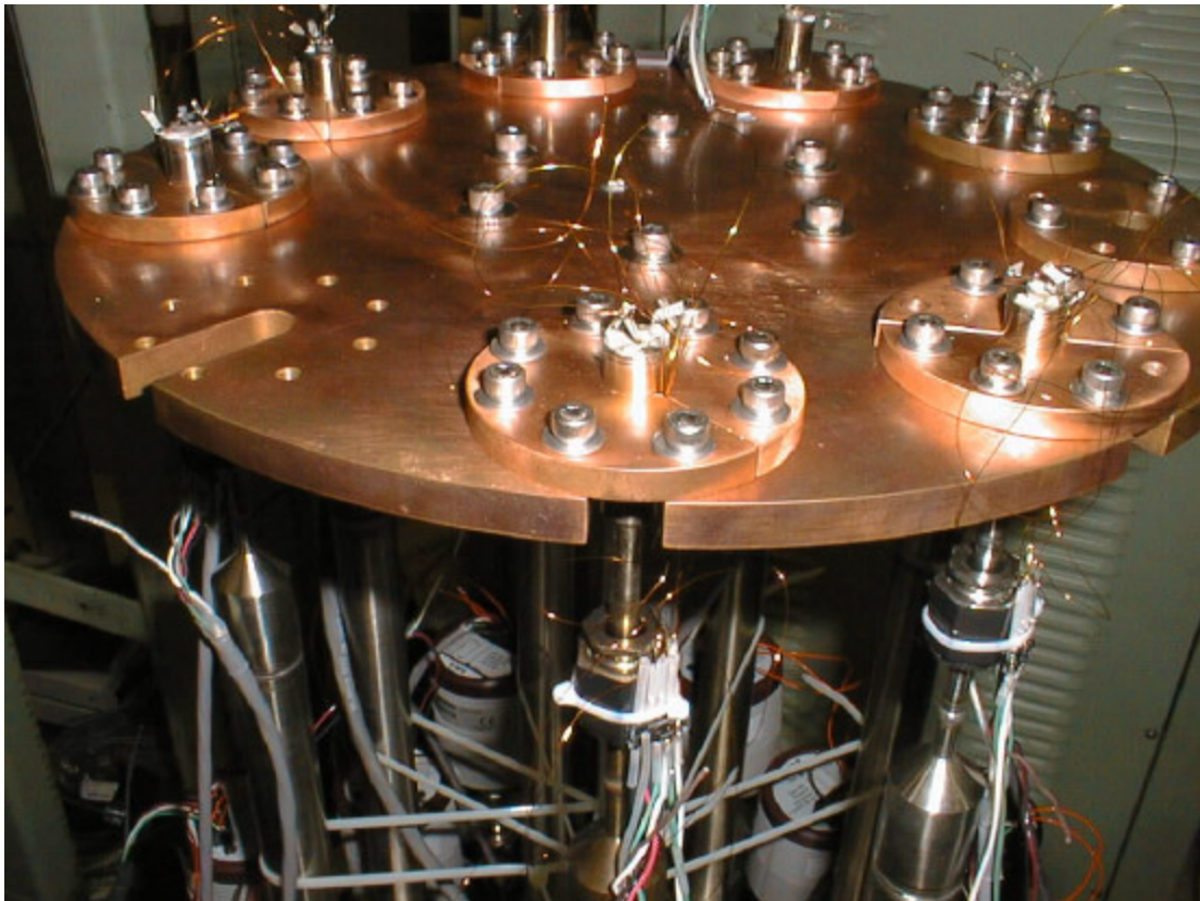
Figure 4-15 Actuator test assemblies in the vacuum chamber.
